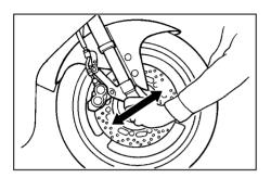
2. Hold the lower ends of the front fork legs and try to move them forward and backward. If any free play can be felt, have a Yamaha dealer check or repair the steering.
